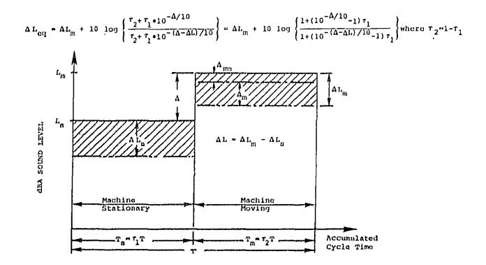
Figure 3-1 EFFECT OF NOISE CONTROL ON WORK CYCLE AL
