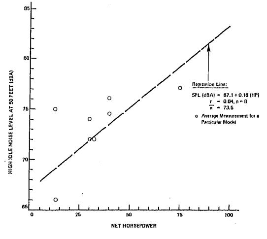
Figure 4-6 HIGH IDLE SOUND LEVEL VS. NET HORSEPOWER FOR SKID STEER LOADERS
