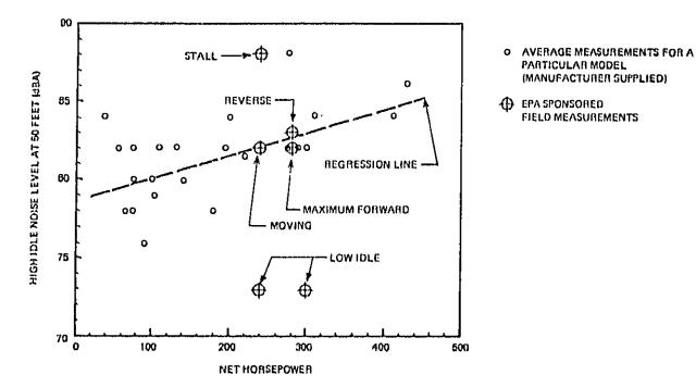
Figure 4-12 Observed Sound Levels at Construction Sites (High Jdle Sound Levels vs. Net Horsepower for Crawler Dozers)
