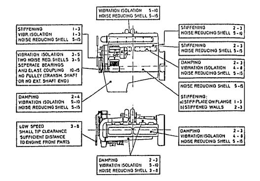
Figure 6-4 WATER-COOLED DIESEL ENGINE, METHODS OF IMPROVEMENT AND EMPIRICAL DATA IN dBA FOR NOISE REDUCTION OF EXTERNAL ENGINE SURFACES
