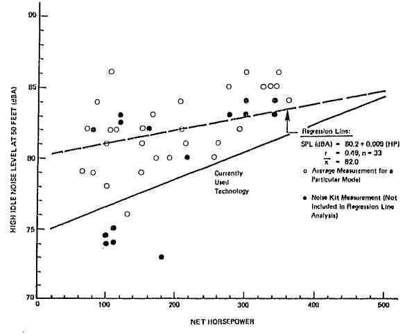
Figure 4-4 HIGH IDLE SOUND LEVEL VS. NET HORSEPOWER FOR WHEEL LOADERS
