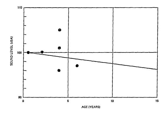
Figure 4-8 Sound Level vs Age for an Individual Crawler Tractor Model
